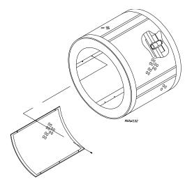
Remove the tumbler and support assembly from the front of the dryer. If the tumbler cannot be removed freely, clean the shaft area and spray WD-40 or similar lubricant. With a block of wood against the shaft end, strike the block of wood with a hammer or mallet to move the shaft past any burrs made by the setscrews.
